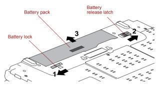
Figure 6-1 Releasing the battery pack
